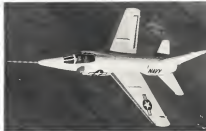
LATEST TIGER , redesignated F11F1, shows larger nose, second canopy and duct inlet and new vertical tail.
